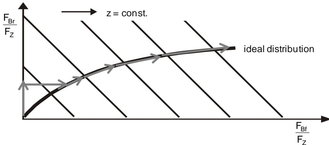
Fig. 10: Schematics Brake Force Distribution
