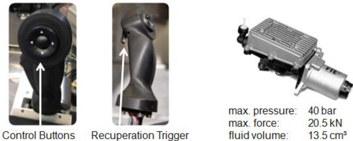
Fig. 6: Sidesticks and Electro Hydraulic Actuator
