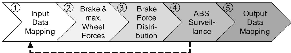
Fig. 9: Brake System Concept
