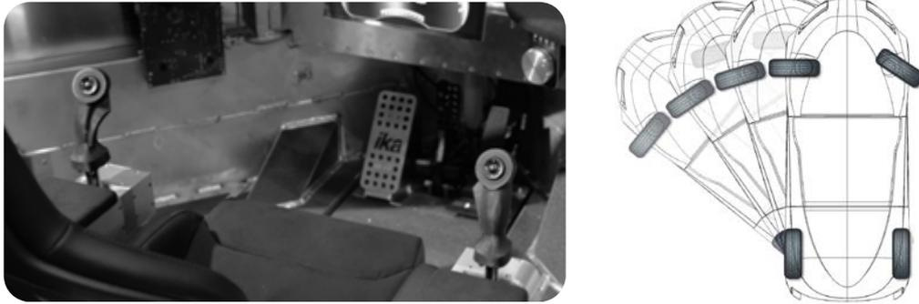
Fig. 3: Steering via sidesticks, high maneuverability
